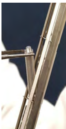
Figure 18: Device for cladding pressure test.
