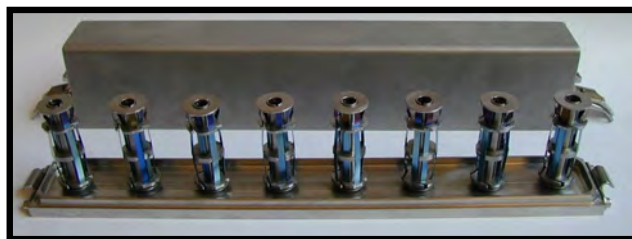
Figure 22: Samples for irradiation bowing tests.
