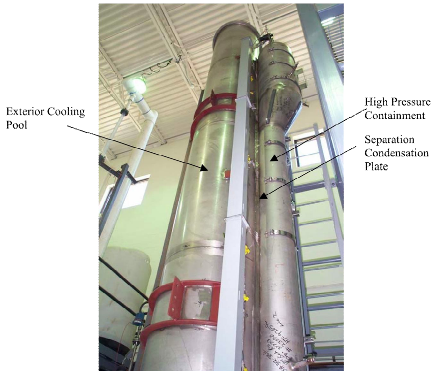
Figure 26 NuScale ITF containment
