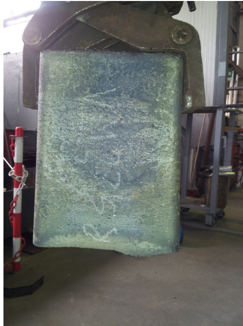
Figure 3 – VIM ingot EP302 stainless steel VM2758
