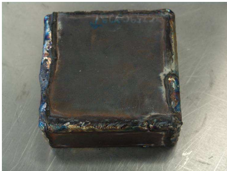
Picture 1. Illustration of block of steel welded metal box to avoid excessive oxidation during heat treatment
