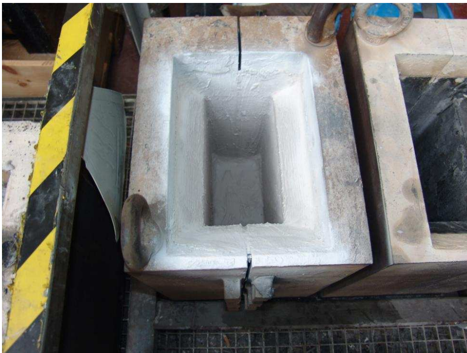
Picture 4. Crucible with protective coating
