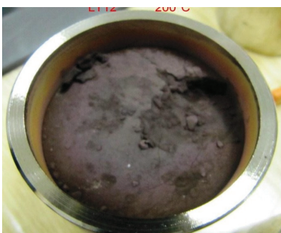
Measurement Tool: Visual Inspection Powder compaction: Total compaction
