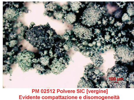
Fig. 77 – Si-C powder - 20°C.
