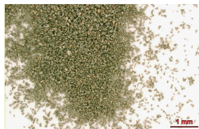
Fig. 81 – Brass powder OT-63 - 500°C.
