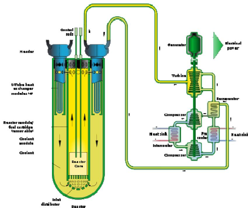
Figure 1 – Sketch of Lead Fast Reactor.
