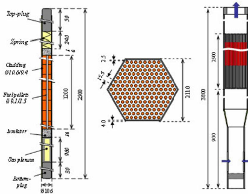
Figure 3 – Schematic view of fuel rod and sub-assembly
