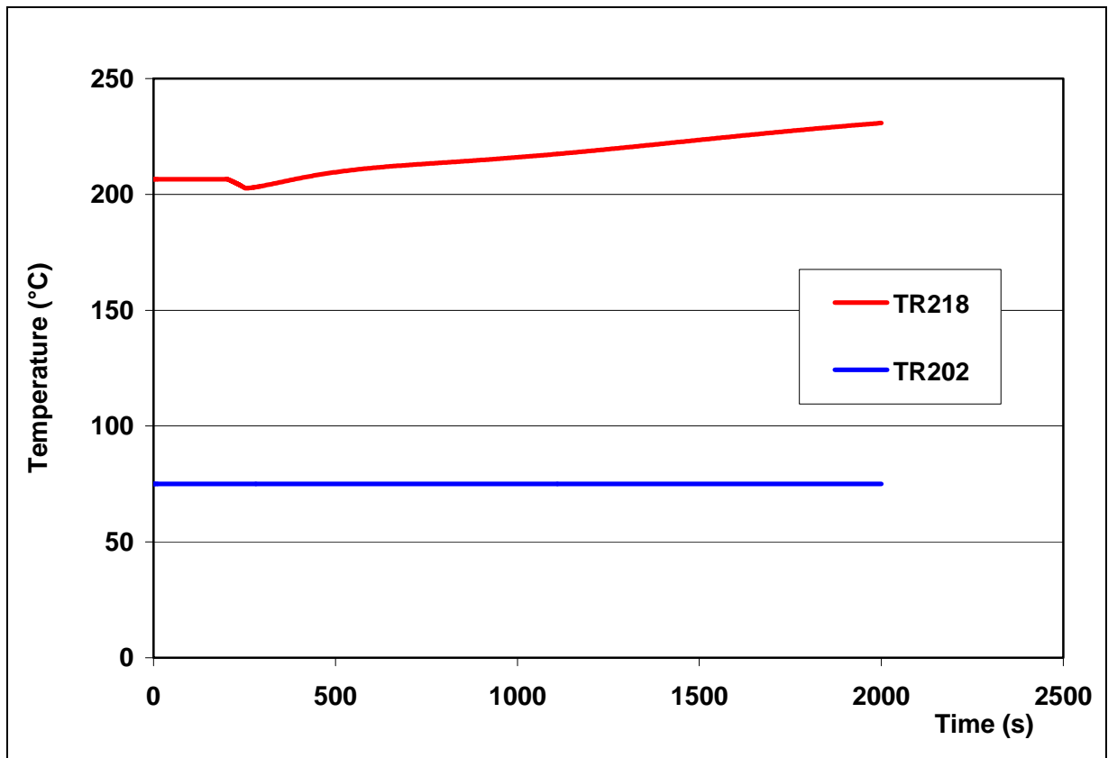
Fig. 4.14 – Inlet and Outlet Air Cooler Temperatures
