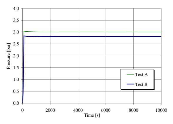
Figure 17. Differential pressure measured through the main pump.
