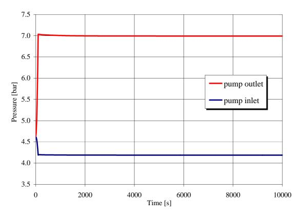
Figure 16. Inlet and outlet pressure in the pump.
