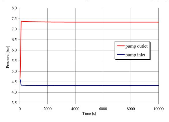
Figure 13. Inlet and outlet pressure in the pump.
