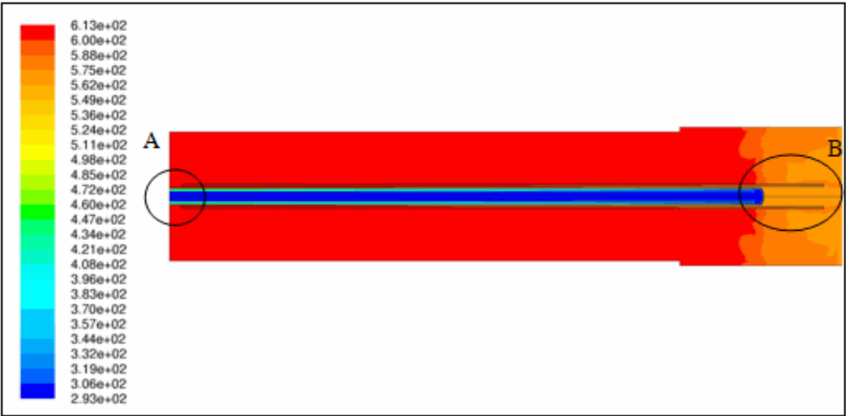
Figure 26. Air temperature contour plot [K]
