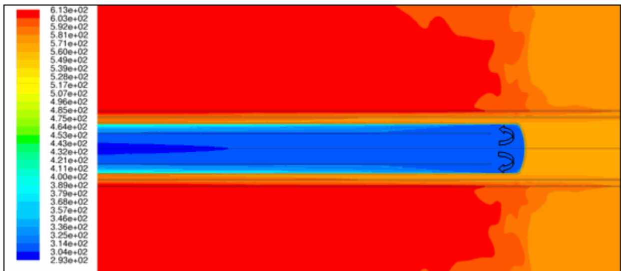
Figure 28. Air temperature contour plot [K] at the end of air pipe (region B)
