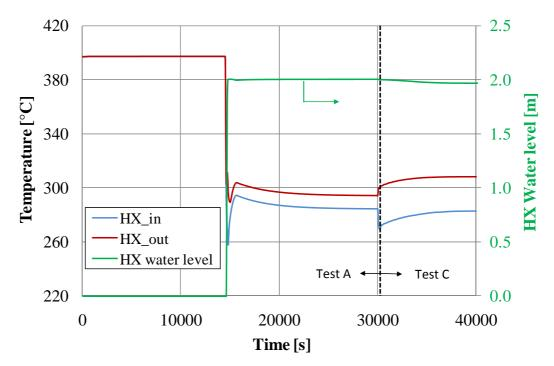
Figure 11. Time trend of the water level and of inlet and outlet temperature through the secondary side of HX (Test A + Test C)
