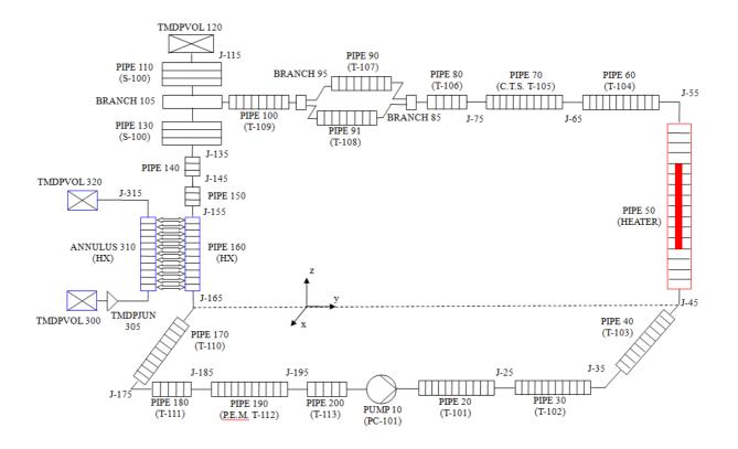
Figure 4. Relap5 nodalization for the primary loop
