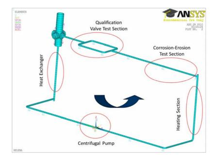
Figure 1. Layout of the primary loop
