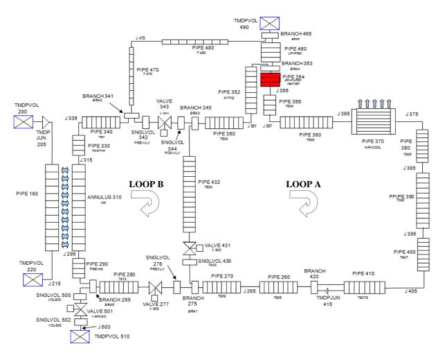
Figure 5. Relap5 nodalization for the secondary loop
