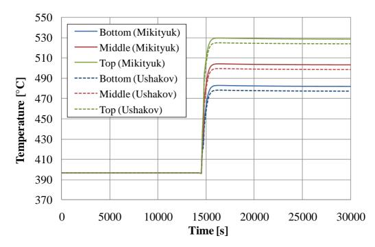
Figure 7. Comparison between wall rod temperatures obtained with the two different correlations in the HS of the primary loop (Test A)
