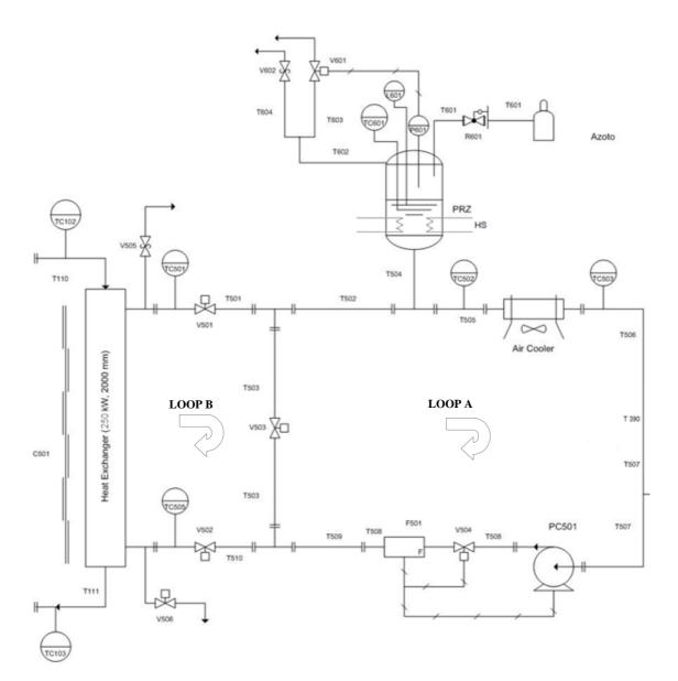
Figure 3. Scheme of secondary loop
