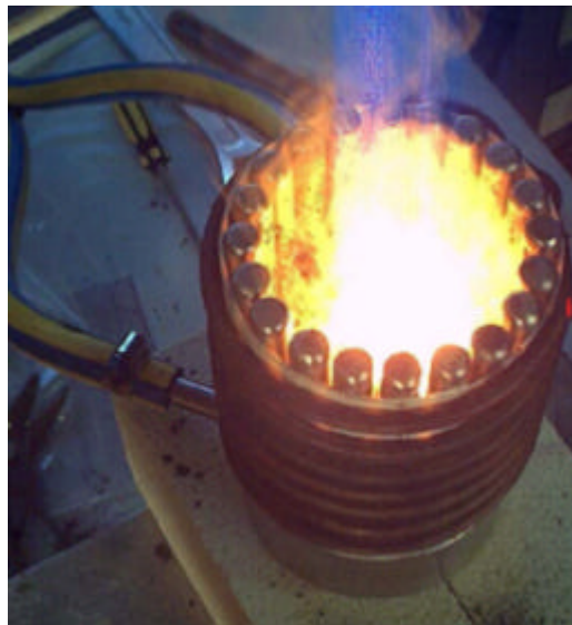
Figura 51 - Fotografie tratte da Internet: Sergey Stefanovsky (SIA Radon, Moscow, Russia), “Cold Crucible Inductive Melting of Vitreous and Ceramic Waste Forms”
