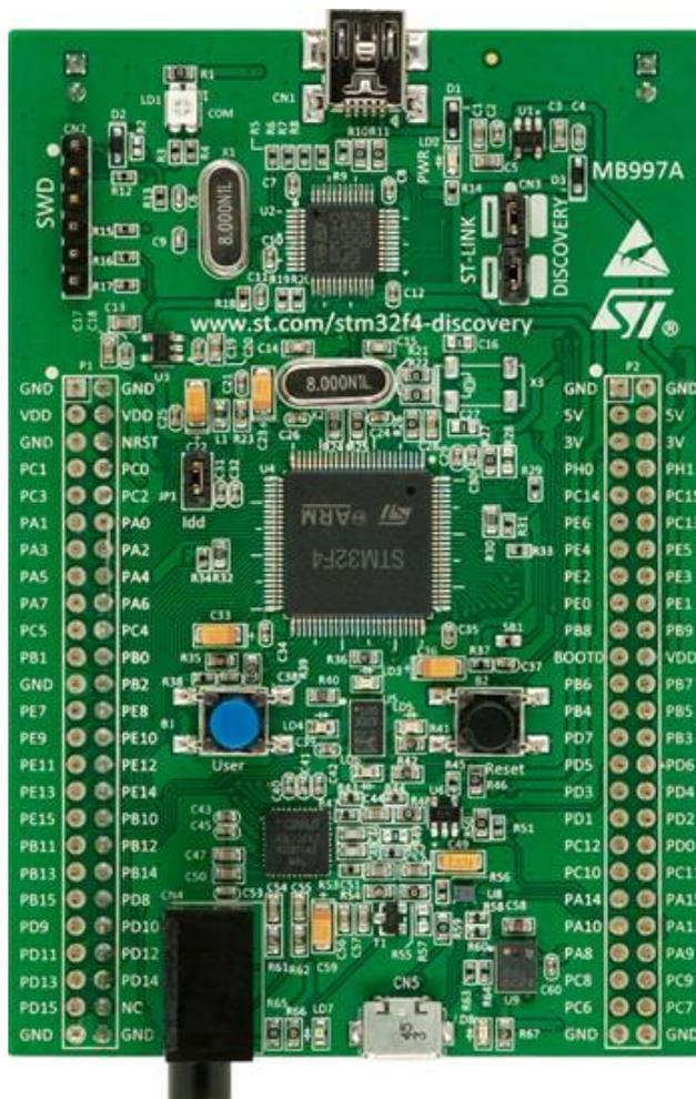
Figura A.56 Discovery kit for STM32 F4 series - with STM32F407VG MCU
