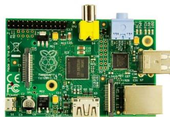
Figura 18: Raspberry Pi Model B
