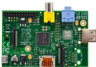
Figura 17: Raspberry Pi Model A
