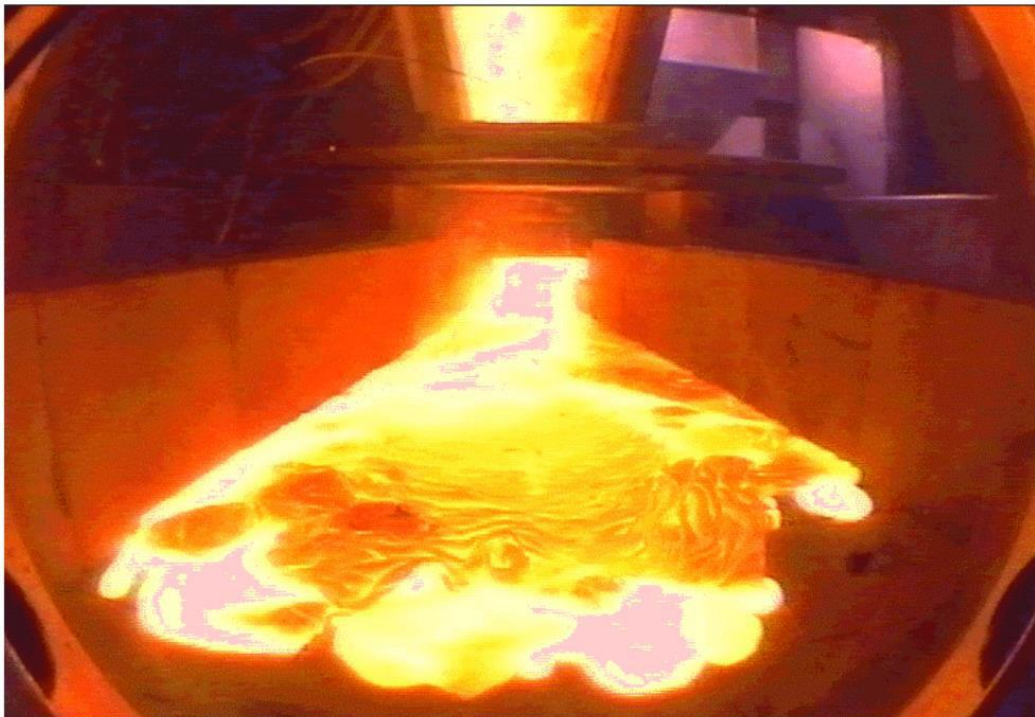
Corium spreading test at the French CEA VULCANO facility (UO 2 with some ZrO 2 ) ( http://www.iaea.org/NuclearPower/Downloads/INPRO/Files/2010-Feb-DF-WS/15-Teller.pdf )
