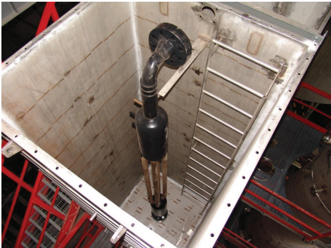
Figure 5 – SPES 3 condenser pool with condenser: inside view
