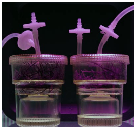
“Hairy Roots” biofermenters for high-value added molecule production
