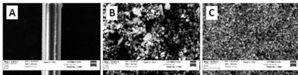
Scanning Electron Microscope images of basalt fibers. A) Whole basalt fiber. B) Fine sized basalt fibers after grinding process. C) Ultra-fine sized basalt fibers after grinding process
