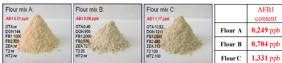
Fig. 2 - Analysis and determination of aflatoxin B1 content in three flours naturally contaminated with different mycotoxins. The AFB1 content of each flour mix, determined by competitive ELISA, are reported in the table as ppb (parts per billions) and matched with the real AFB1 content, determined by chemical analysis (HPLC). The data are the mean of three technical replicates and have been elaborated with a commercial software.
