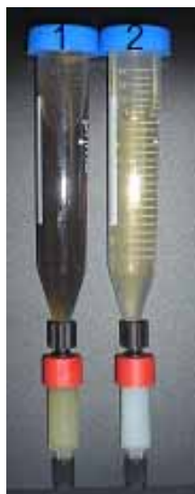
Fig. 2 - Visual comparison between clarified total extract from fresh Agro-infiltrated leaves obtained by mechanical homogenization (1) or intercellular fluids (IFs) (2). In the bottom part, protein A chromatography columns after three purification cycles from the corresponding extracts are shown. Extraction procedure, based on the recovery of IFs, gave purification yields of 15\text{-}20 \text{ mg} / \text{Kg FW} (corresponding to 27% of total soluble protein) with a total phenolic compounds content reduced by one order of magnitude ( 21 \mu\text{g} / \text{g FW} ) compared to total extract.
