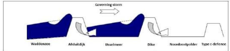
Figure 2.10: Schematization of the IJsselmeer water system during a breach in the Afsluitdijk
