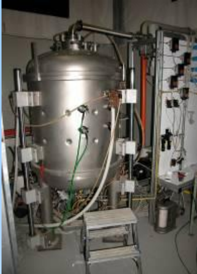
Impianto CVI in FN
