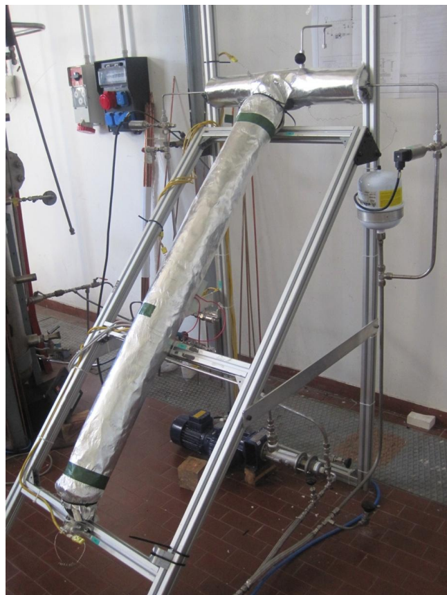
Impianto T.O.S.C.A. (Thermal fluid dynamics Of Solar Cooling Apparatus)
