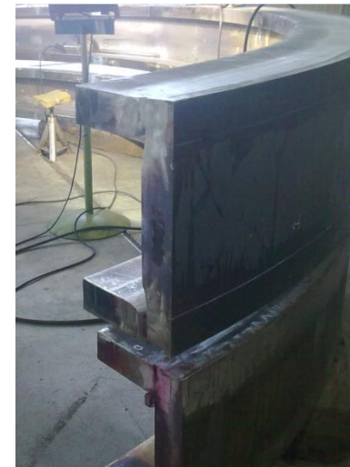
Gambe curve saldate EBW
